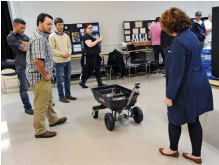
From left, Ellison Stancil , Brady Morton , and Luke Martin demonstrate their Companion Wheelbarrow to Mandy Orzechowski , dean of the Engineering and Industrial Technology Division, right. The wheelbarrow follows the operator—requiring no work for the owner, besides loading the wheelbarrow.
